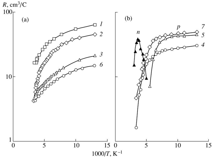
**Fig. 3.** Temperature dependences of the Hall coefficient  $R$  for samples with various In content  $X$  in the GaInAsSb solid solution. (a) Samples with a high mobility at  $T = 77$  K and (b) samples with a low mobility at  $T = 77$  K. Curve numbers correspond to sample numbers in Table 2.
